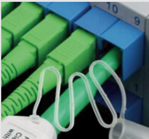
Cleaning of SC connectors (also FC and ST)
